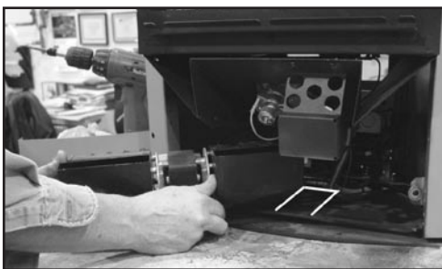
Figure 8.28 Slide the blower into the bracket as indicated. Ensure the blower is pushed back into the bracket to allow the replacement of the lower access door. The magnet strips located on the blower feet are designed to hold the blower in place.
