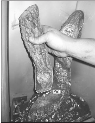
Figure 8.17 Locate log #2 over the pin in log #1 and into notch in log #1. Lean the log back toward the left corner of the firebox.
